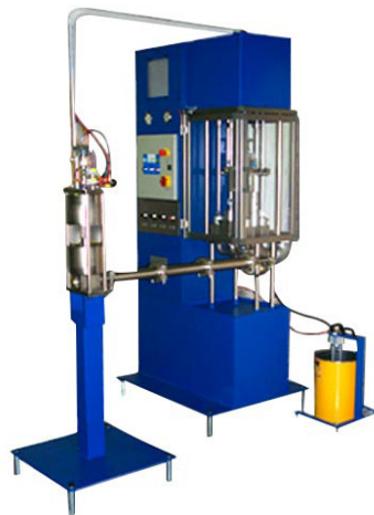
Static mixer for coloring or catalyzing any basic product.
