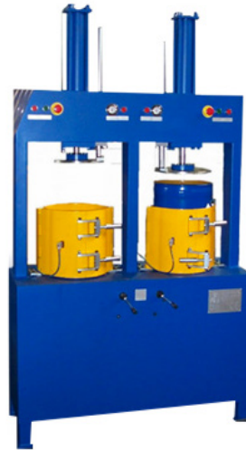
Extruder for pails/buckets with double pressing plate , with a single hydraulic cylinder for the simultaneous lowering of both pressing plates or with two hydraulic cylinders for independent lowering of each pressing plate.
